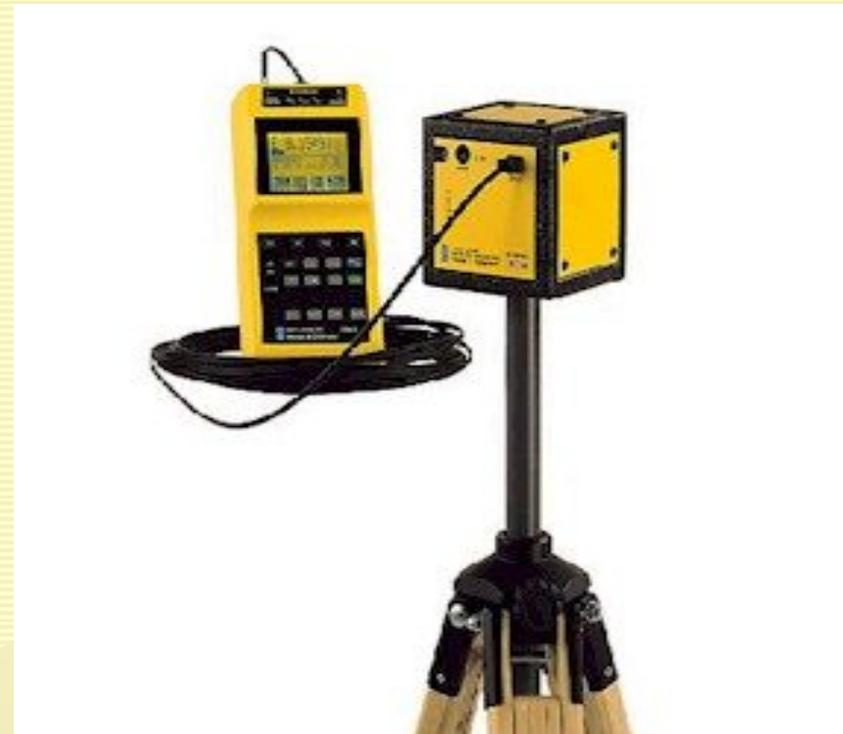
***FIG. 6. Electromagnetic field analyzer and its electric field probe***
